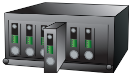
Figure 3-2: Insert a video over fiber converter into an available slot
