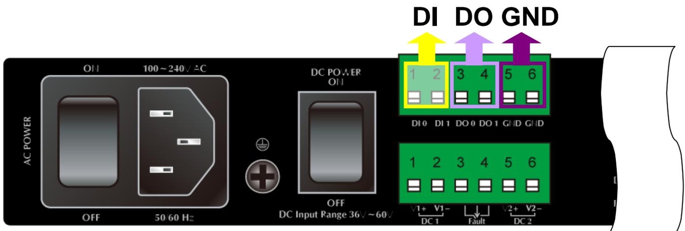
Figure 2-1-9 Wiring the Redundant Power Inputs
