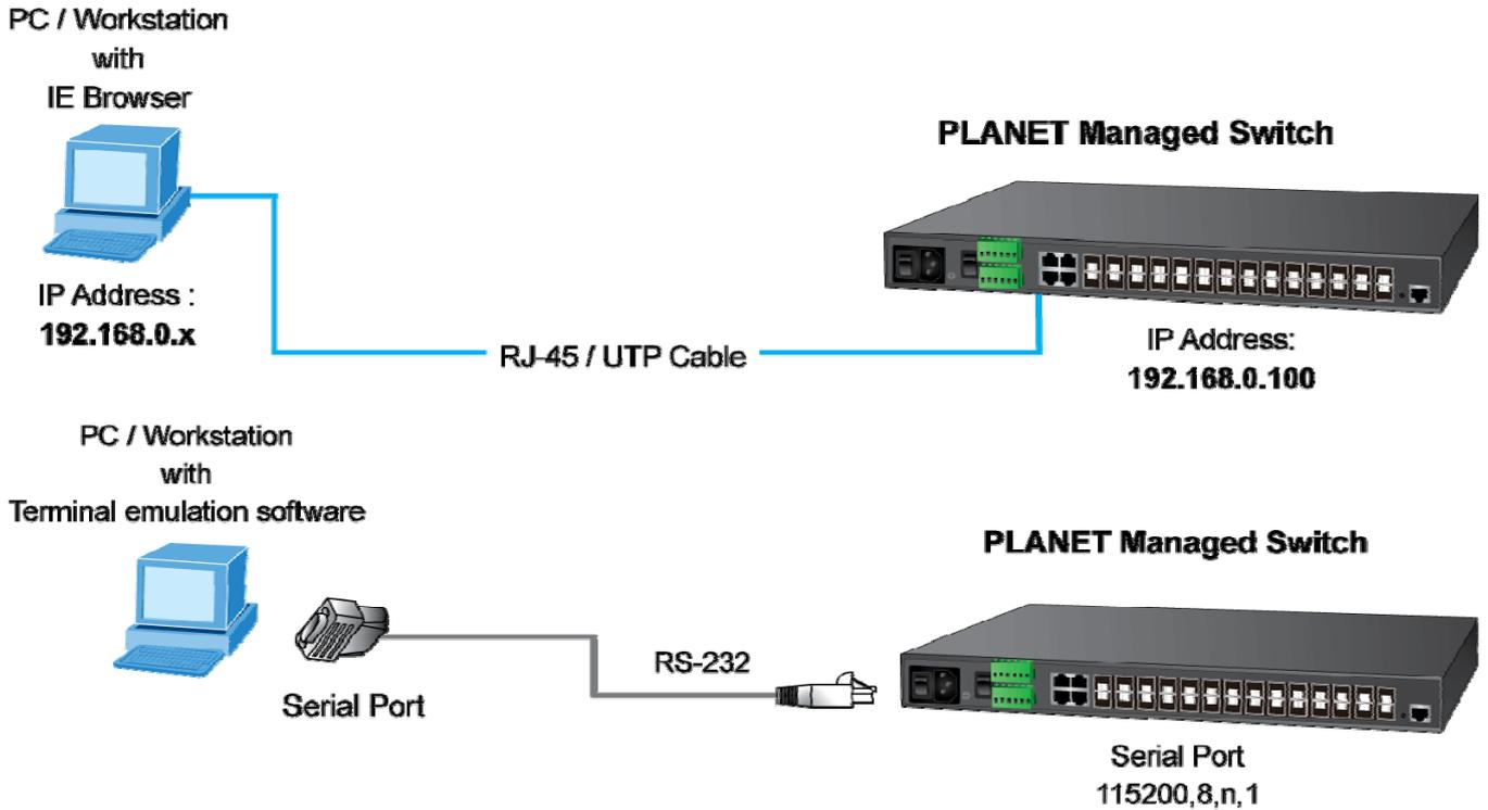
Figure 3-1: Remote Telnet and Console Port Interface Management
