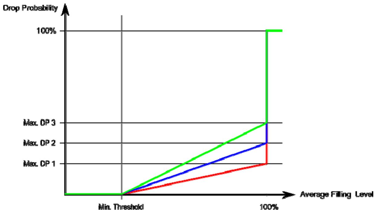
This page allows you to configure the Random Early Detection (RED) settings for queue 0 to 5. RED cannot be applied to queue 6 and 7. Through different RED configuration for the queues (QoS classes) it is possible to obtain Weighted Random Early Detection (WRED) operation between queues. The settings are global for all ports in the switch. The QoS Statistics screen in [Figure 4-9-16](#) appears.
