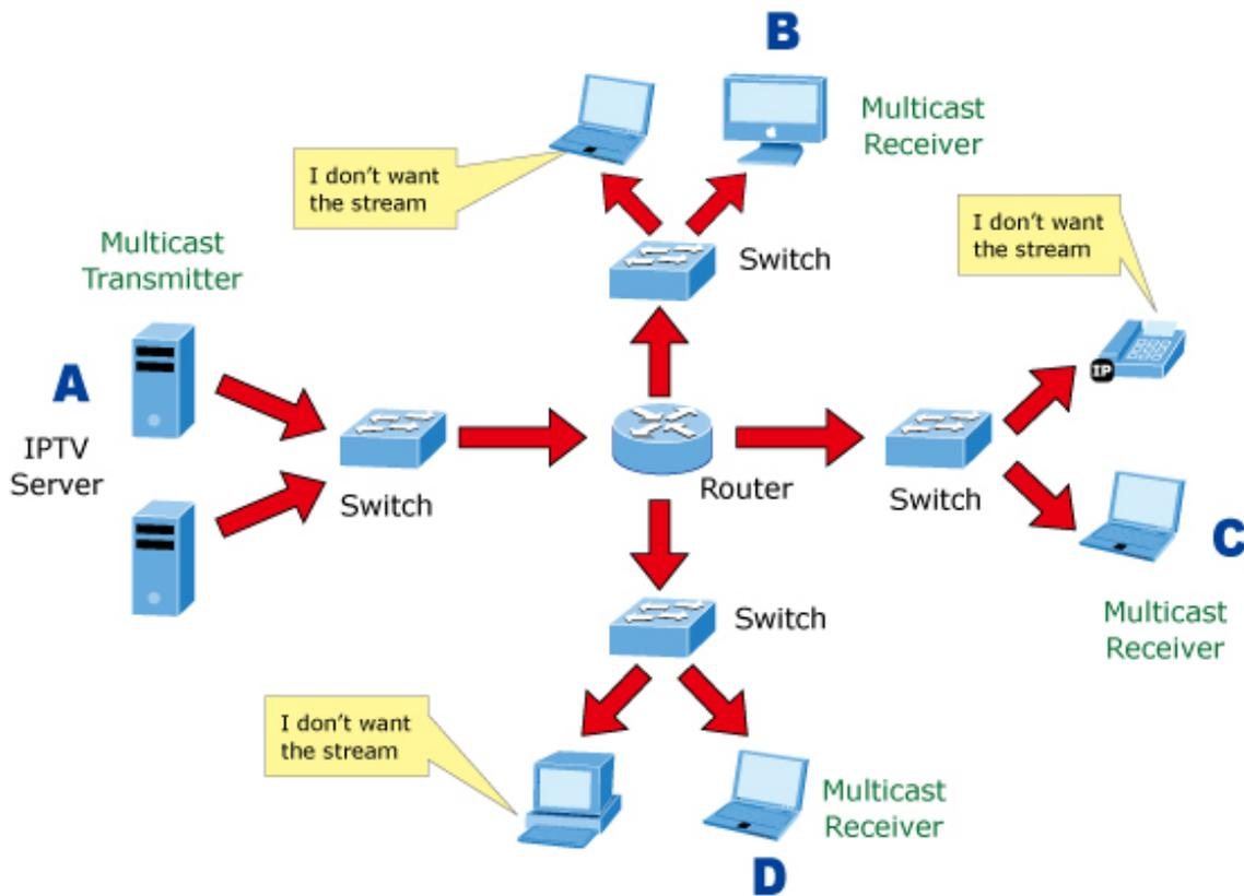
Figure 4-8-2: Multicast Flooding
