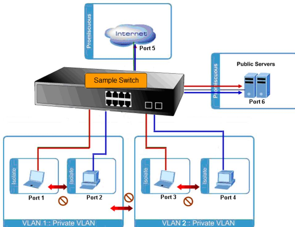
Figure 4-6-16: The Port Isolate VLAN Diagram
