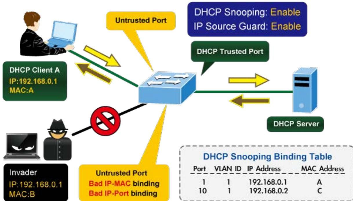
This page provides IP Source Guard related configuration. The IP Source Guard Configuration screen in [Figure 4-12-10](#) appears.
