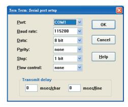
Figure 4-2 Tera Term COM Port Configuration
