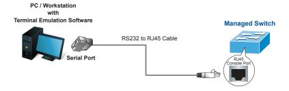
Figure 4-1 Managed Switch Console Connectivity
