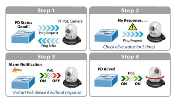
This page provides you with how to configure PD Alive Check. The screen in Figure 4-7-7 appears.
