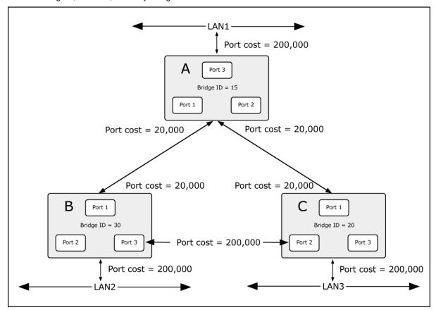
Figure 4-3-55: Before Applying the STA Rules
