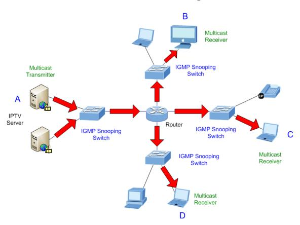
**IGMP Snooping Multicast Stream Control**
