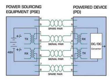
Figure 8-2: Power Supplied over the Data Pins
