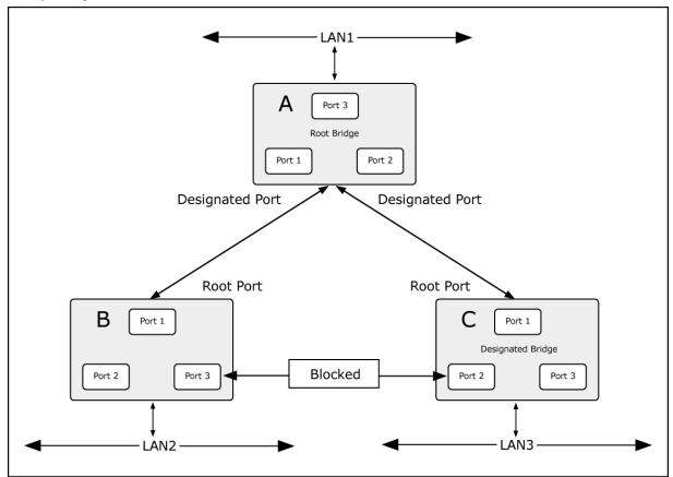
Figure 4-3-56: After Applying the STA Rules
