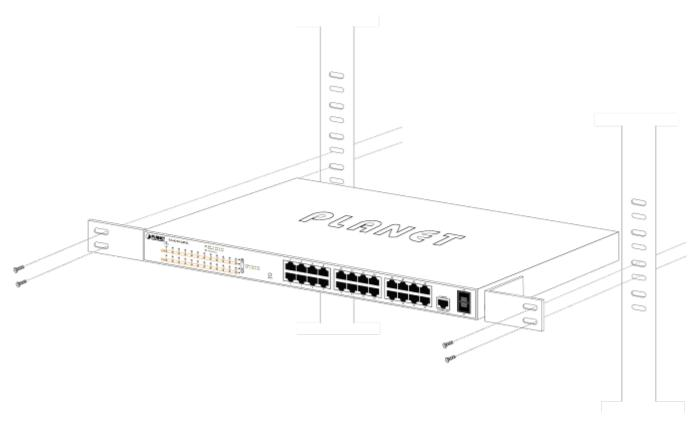
Figure 2-1-31: Mounting Managed Switch in a Rack
