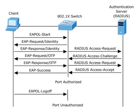
Figure 4-5-24: EAP Message Exchange
