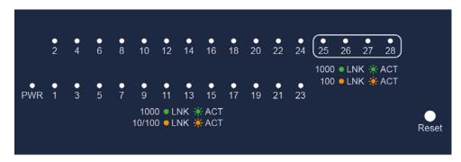
Figure 2-1-16: GS-4210-24T4S(R) LED Panel
