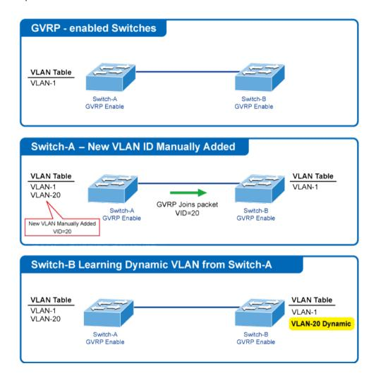
VLANs are **dynamically** configured based on **join messages** issued by host devices and propagated throughout the network.
