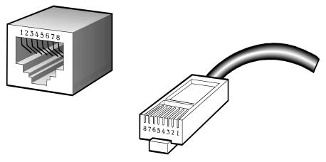
The standard RJ45 receptacle/connector
