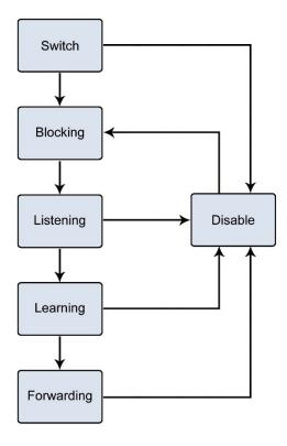
Figure 4-3-54: STP Port State Transitions
