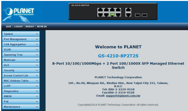
Figure 8-3: Web Main Screen of Managed Switch
