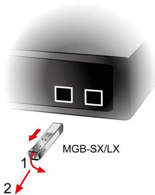
Figure 2-1-8 How to Pull Out the SFP Transceiver
