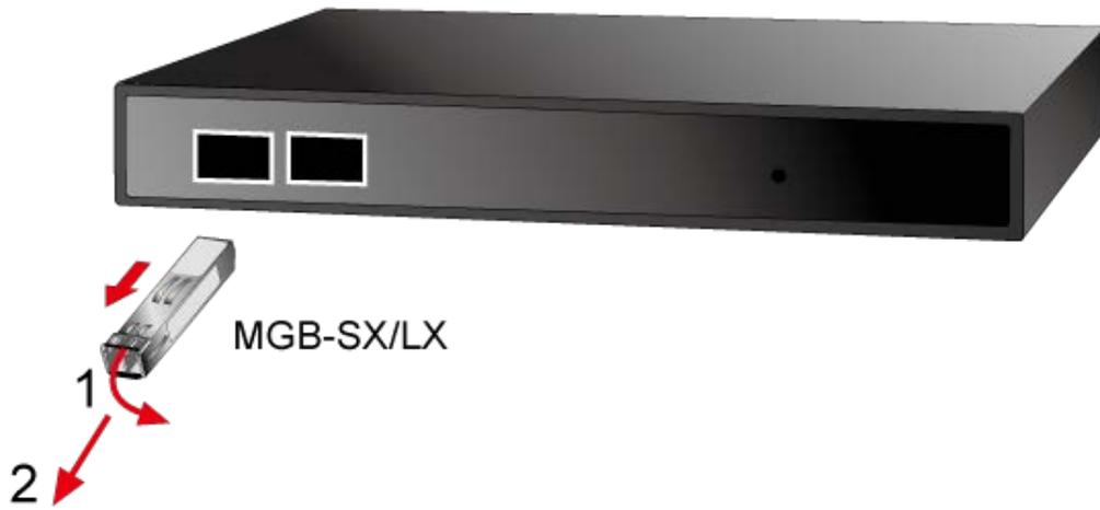
**Figure 2-8** How to Pull Out the SFP Transceiver
