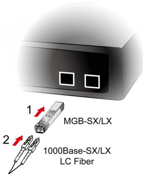
Figure 2-8: Plugging in the SFP Transceiver
