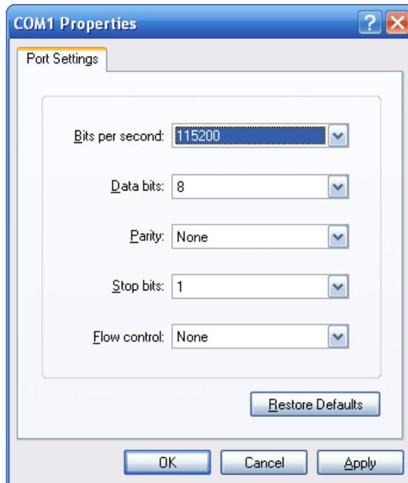
**Figure 5-3** Hyper Terminal COM Port Configuration
