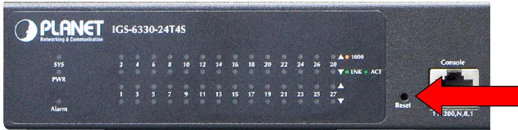
Figure 2-2: Reset button of Industrial Managed Switch
