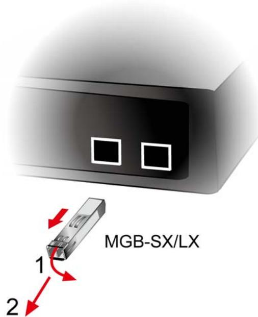
**Figure 2-9:** Pulling out the SFP Transceiver Module
