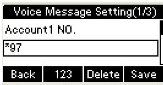
6. Press the OK key on the phone keyboard or the Save soft key to save and return to message interface.
