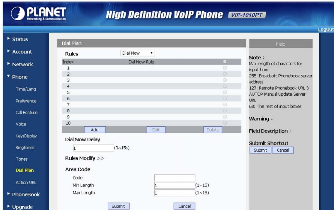
The screenshot shows the 'Dial Plan' configuration page. The 'Rules' table has a 'Dial Now' dropdown menu. Below the table are 'Add', 'Edit', and 'Delete' buttons. The 'Dial Now Delay' section has an input box set to '1' with '(0~15s)' next to it. The 'Rules Modify >>' section includes an 'Area Code' field and 'Min Length' and 'Max Length' input boxes, both set to '1'. A 'Submit' button is at the bottom.
