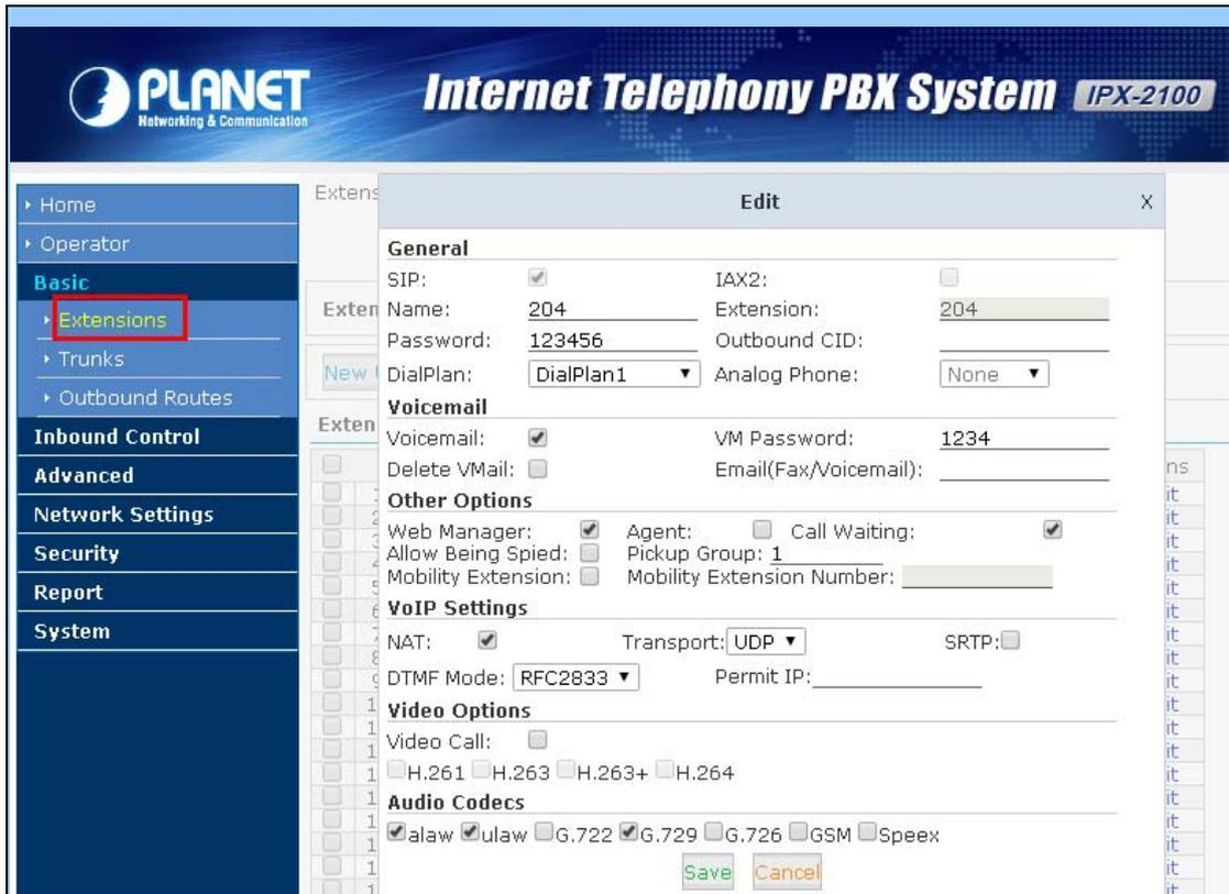
The screenshot shows the PLANET IPX-2100 web interface. The left sidebar has a menu with 'Basic' expanded to 'Extensions'. The main content area shows an 'Edit' window for extension 204. The fields are as follows:
