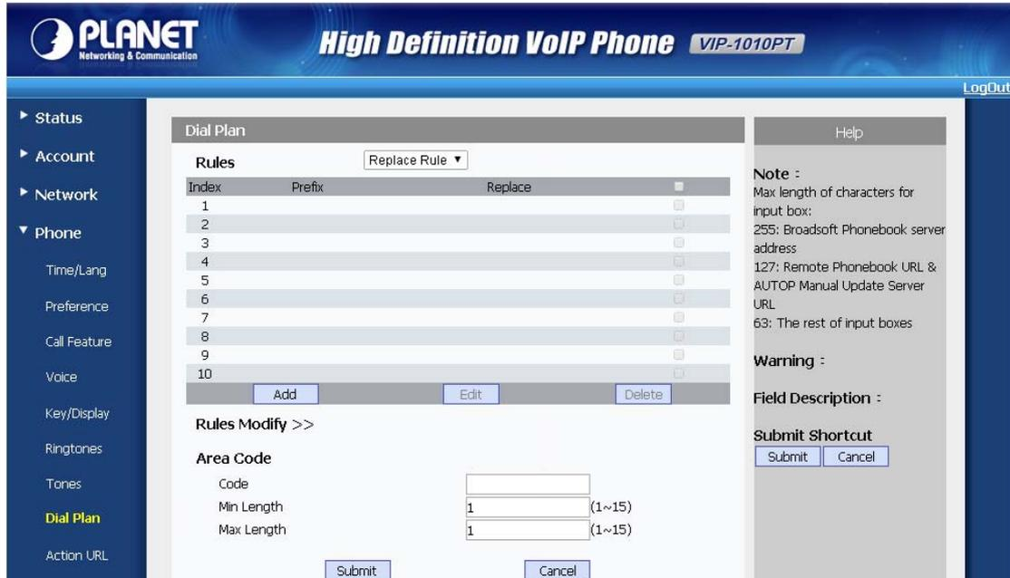
The screenshot shows the 'Dial Plan' configuration page. The 'Rules' table has a 'Replace Rule' dropdown menu. Below the table are 'Add', 'Edit', and 'Delete' buttons. The 'Rules Modify >>' section includes an 'Area Code' field and 'Min Length' and 'Max Length' input boxes, both set to '1'. A 'Submit' button is at the bottom.
