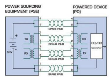
Figure 8-1: Power Supplied over the Spare Pins
