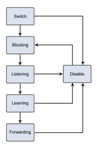
Figure 4-9-2: STP Port State Transitions
