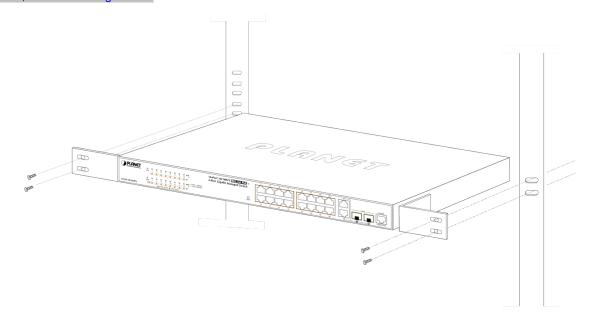
Figure 2-6: Mounting Managed PoE+ Switch in a Rack
