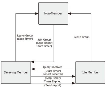
Figure 4-9-16: IGMP State Transitions
