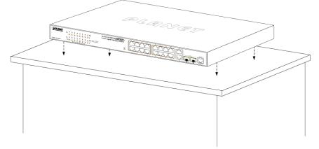
Figure 2-4: Place the Managed PoE+ Switch on the Desktop
