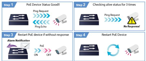
This page provides you with how to configure PD Alive Check. The screen in Figure 4-5-5 appears.
