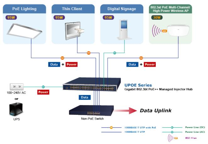
Figure 2-2-4: Network application installation
