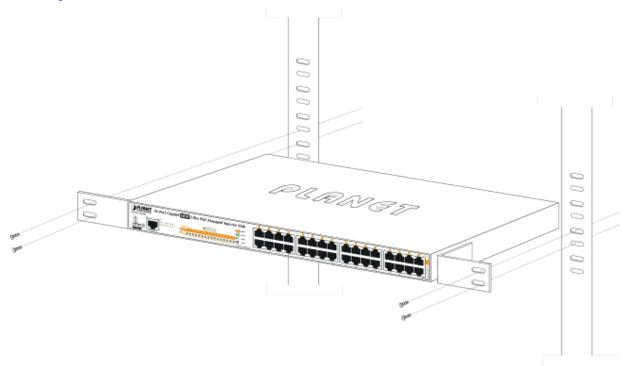
Figure 2-2-3: Mounting the 802.3bt PoE++ Managed Injector Hub in a Rack
