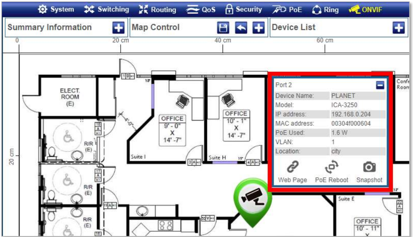
Figure 4-8-1-6: Floor Map Page Screenshot – Display device information of selected ONVIF IP camera
