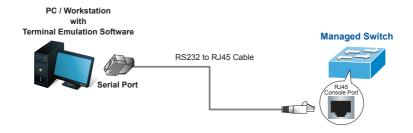
Figure 4-1 Managed Switch Console Connectivity
