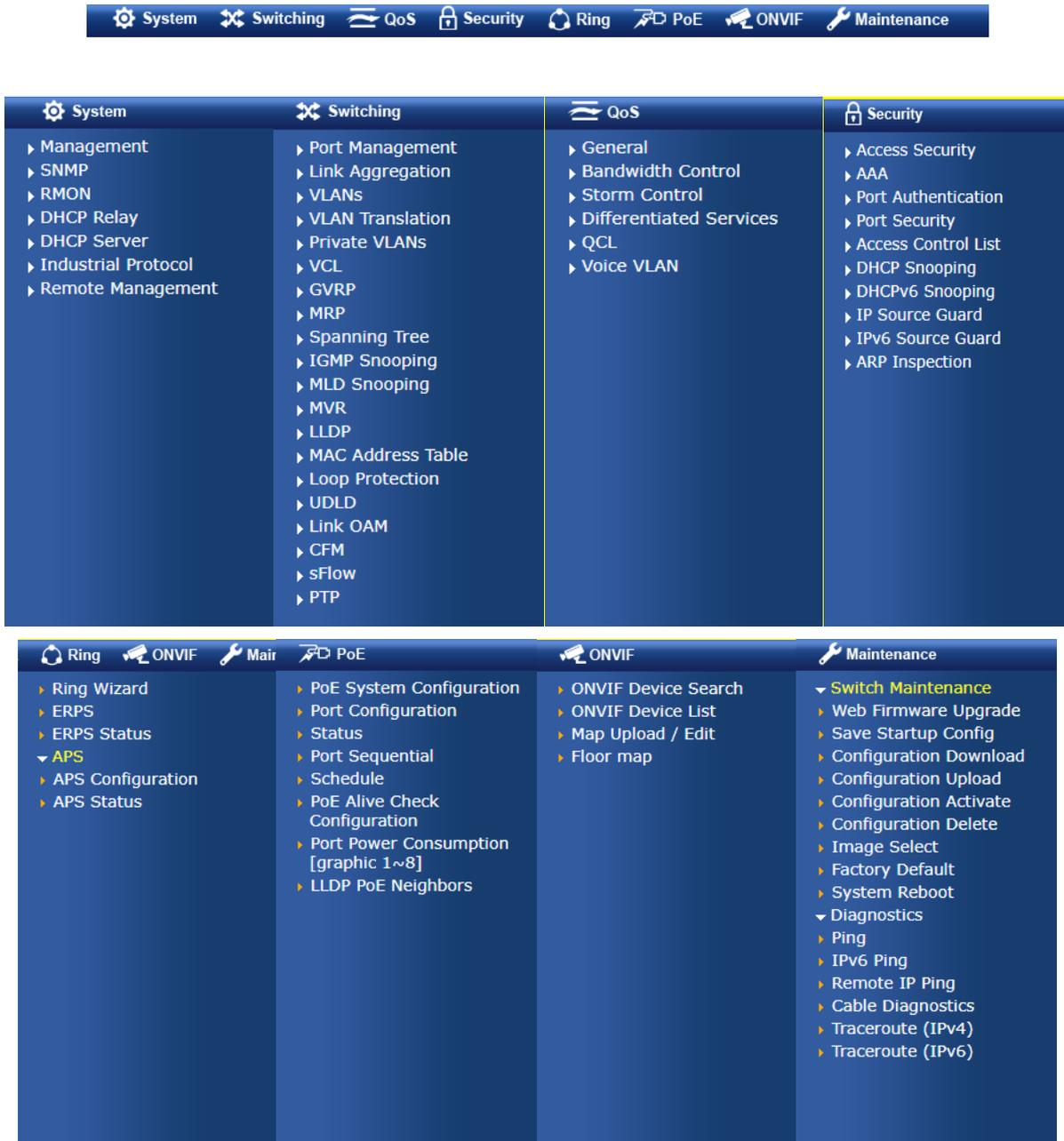
Figure 4-1-5: Wall-mount Managed Switch Main Functions Menu
