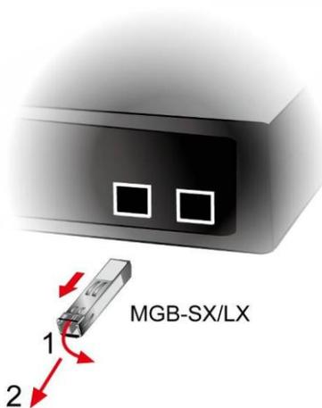
Figure 2-2-5: How to Pull Out the SFP Transceiver
