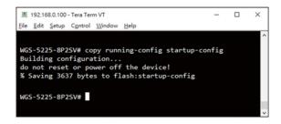
Figure 6-3: Saving Current Configuration Command Screen
