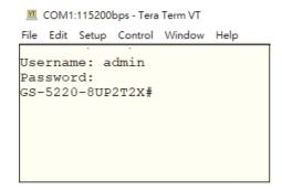
Figure 3-3: Managed PoE Switch Console Login Screen
