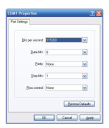
Figure 3-2: COM Port Configuration
