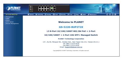
Figure 4-3: Web Main Screen of Managed PoE Switch
