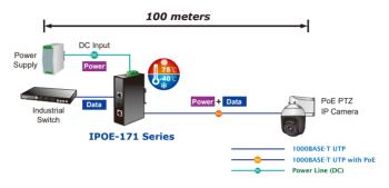
Figure 9: Architecture of connected IEEE 802.3at/bt device
