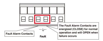
Figure 8: Fault Alarm Contact
