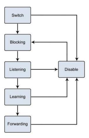
Figure 4-3-4-1: STP Port State Transitions
