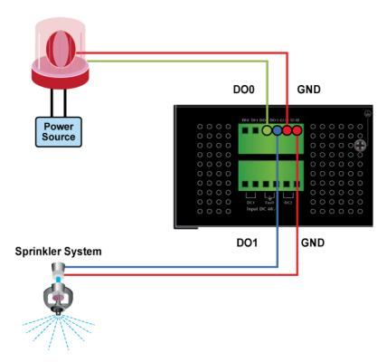
Figure 2-1-16 Wires DO0 and DO1 to Open Detector
