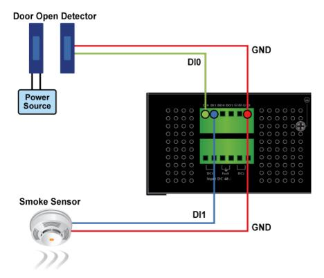
Figure 2-1-15 Wires DI0 and DI1 to Open Detector
