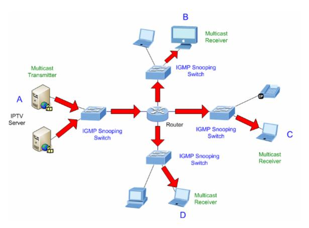
Figure 4-3-5-3: IGMP Snooping Multicast Stream Control
