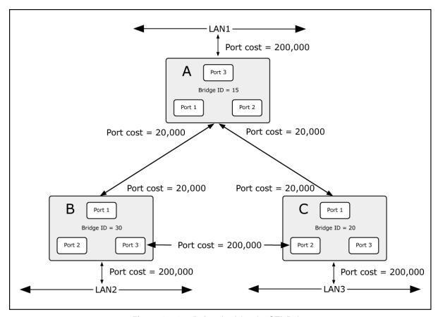
Figure 4-3-4-2: Before Applying the STA Rules
