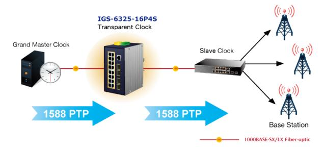
PTP was originally defined in the **IEEE 1588-2002** standard, officially entitled "Standard for a Precision Clock Synchronization Protocol for Networked Measurement and Control Systems" and published in 2002. In 2008 a revised standard, **IEEE 588-2008** was released. This new version, also known as PTP Version 2, improves accuracy, precision and robustness but is not backwards compatible with the original 2002 version.
