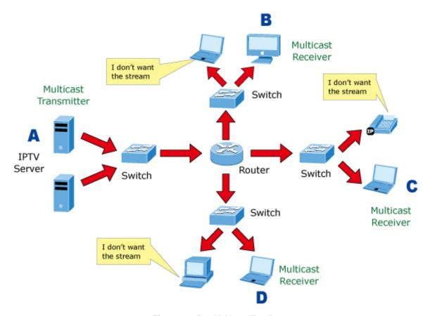
Figure 4-3-5-2: Multicast Flooding
