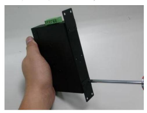
Step 3: Use the screwdriver to screw the wall-mount plate on the Industrial Managed Switch.
