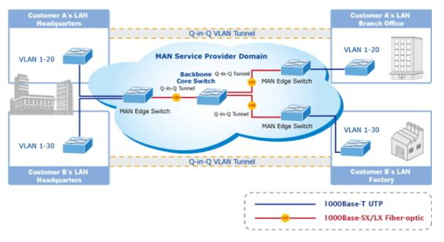
The Industrial Managed Switch supports multiple VLAN tags and can therefore be used in MAN applications as a provider bridge, aggregating traffic from numerous independent customer LANs into the MAN (Metro Access Network) space. One of
