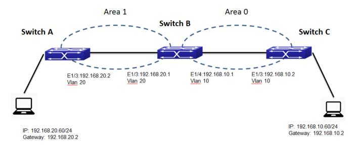
Figure 4-10-4-13 Network topology of OSPF autonomous system
