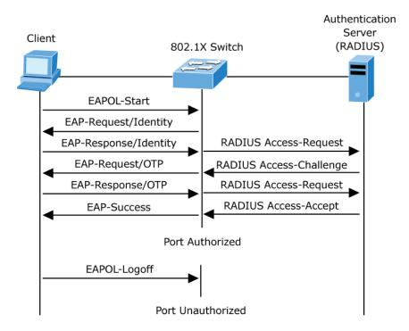
Figure 4-5-2-2: EAP Message Exchange
