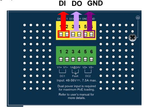
Figure 2-1-13 Wiring the DI and DO of IGS-6325-20T4C4X and IGS-6325-20S4C4X
