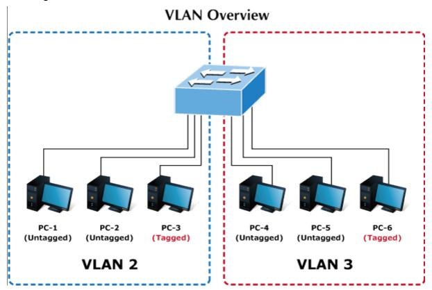
Figure 4-3-3-7: Two Separate VLANs Diagram
