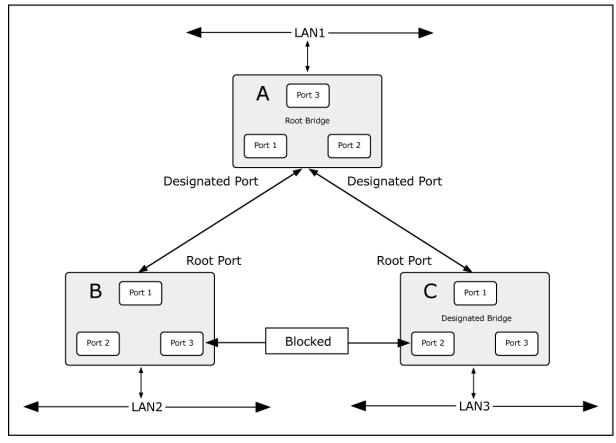
Figure 4-3-4-3: After Applying the STA Rules
