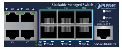
Figure SGS-6310-48T6X front panel
