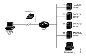
Figure 1-1 Typical AAA Network Configuration
