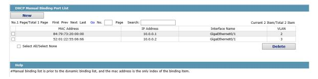
If a host does not obtain the address through DHCP, you can add the binding item on an interface of a switch to enable the host to access the network. You can run no ip source binding MAC IP to delete items from the corresponding binding list.
