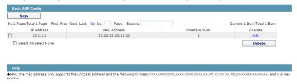
Figure 17 D isplaying static ARP
