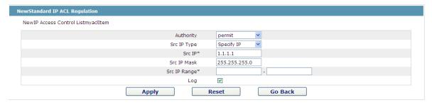
Figure 12: Setting the Rules of the standard IP access control list
