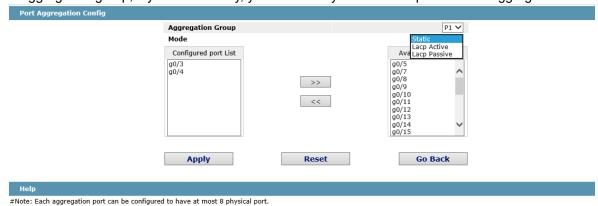
An aggregation group is selectable when it is created but is not selectable when it is modified.
