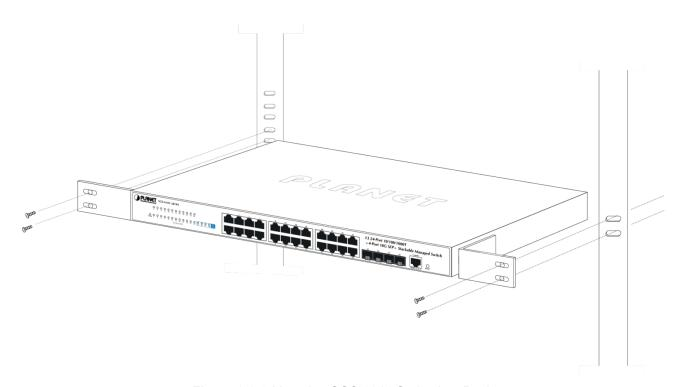
Figure 2-2-3 Mounting SGS-6341 Series in a Rack
