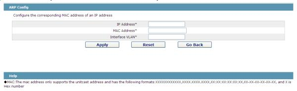
Figure 18 Setting static ARP
