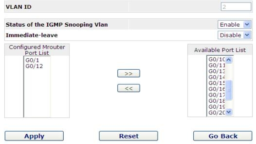
Figure 14: Static routing port of IGMP VLAN
