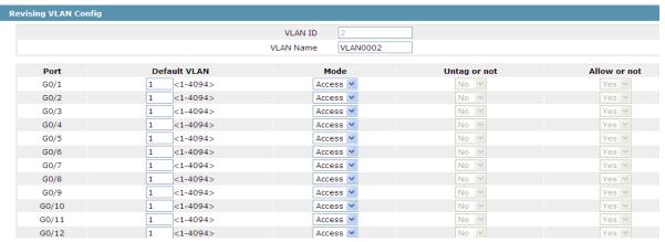
Figure 3 Revising VLAN configuration
