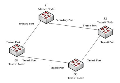
Figure 1.1 EAPS Ethernet ring
