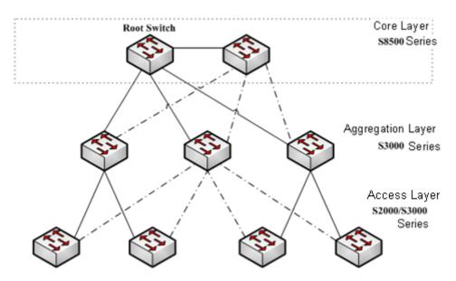
Figure 1.2 Switching network topology
