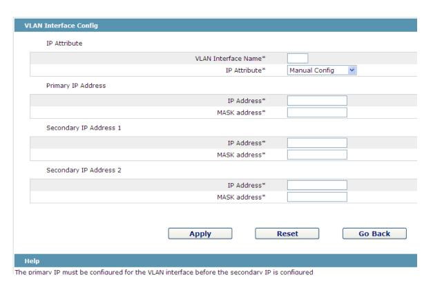
Figure 3: VLAN interface configuration
