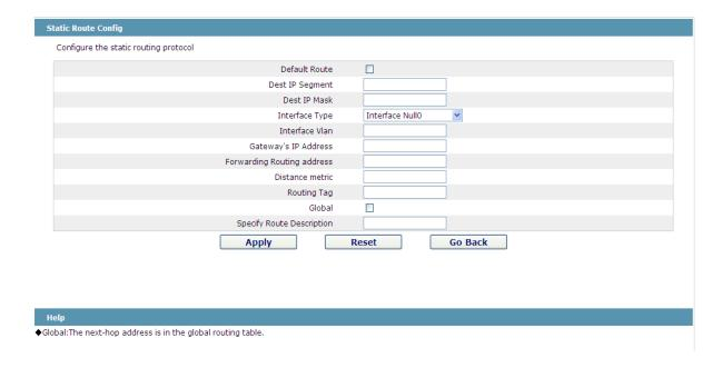
Figure 5: Setting the static route
