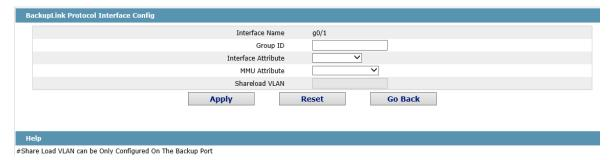
The backup link group which has configured the primary port cannot take other ports as its primary port. Likewise, the backup link group which has configured the backup port cannot take other ports as its backup port.
