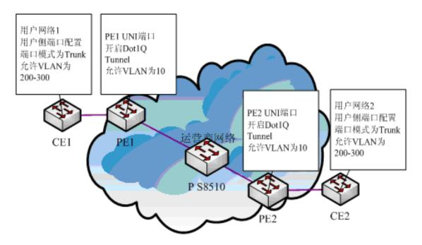
Figure 4 Typical configuration of Dot1Q tunnel
