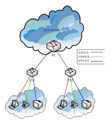
Figure 8 Typical configuration of Dot1Q tunnel (3)
