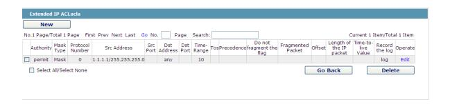
Figure 13: Extended IP access control list
