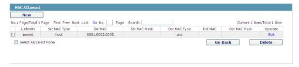
Figure 6: Specific MAC access control list configuration
