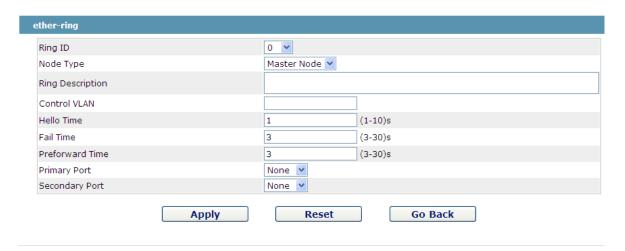
Figure 20 EAPS ring configuration
