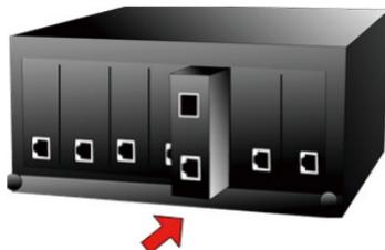
**Step 3:** Attach a rack-mount bracket to each side of the Converter Chassis with supplied screws attached to the package.
