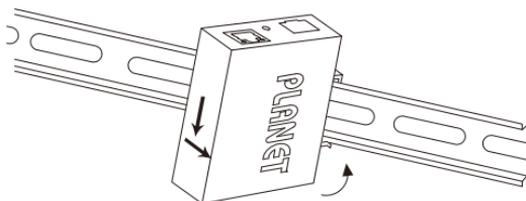
**Step 3:** Check whether the DIN rail is tightly on the track.
