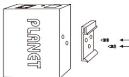
**Step 2:** Now slide the DIN rail into the track.
