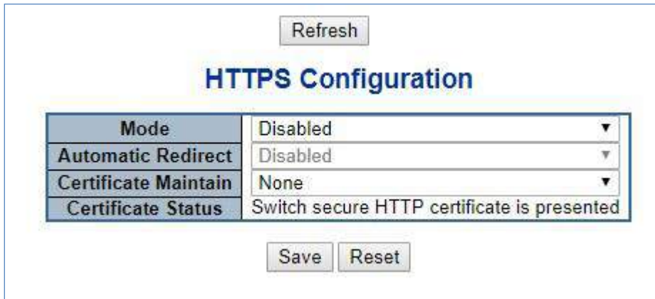
Figure 4-5-1-4: HTTPS Configuration Screen Page Screenshot
