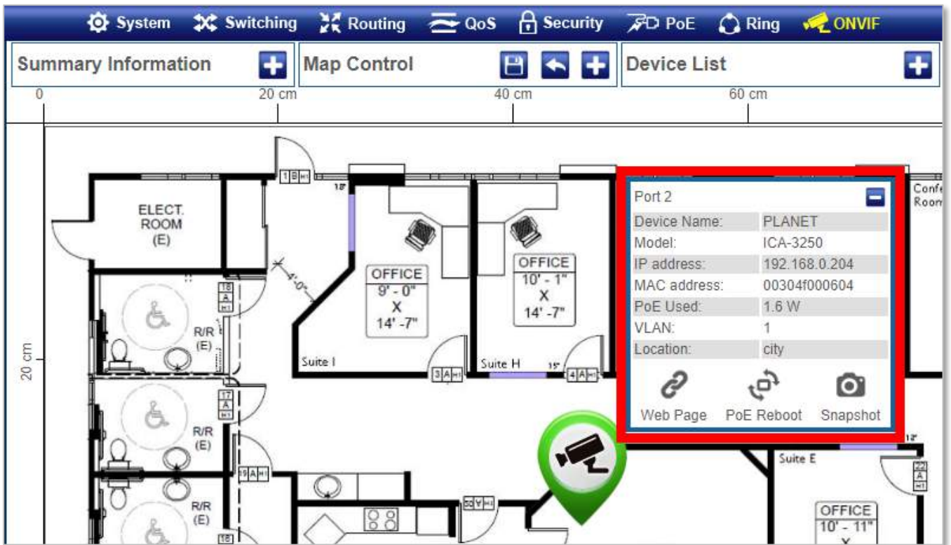
Figure 4-9-1-5: Floor Map Page Screenshot – Display device information of selected ONVIF IP camera
