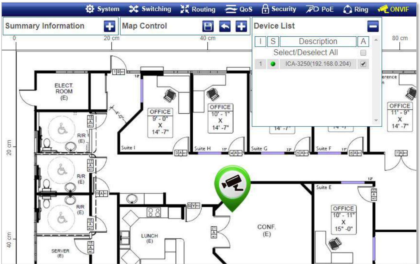
Figure 4-9-1-5: Floor Map Page Screenshot – add ONVIF IP camera from Device List
