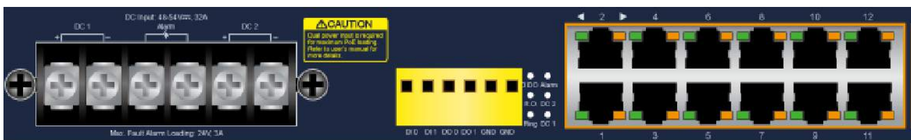
Figure 2-1-16: IGS-6325-24UP4X LEDs on Front Panel
