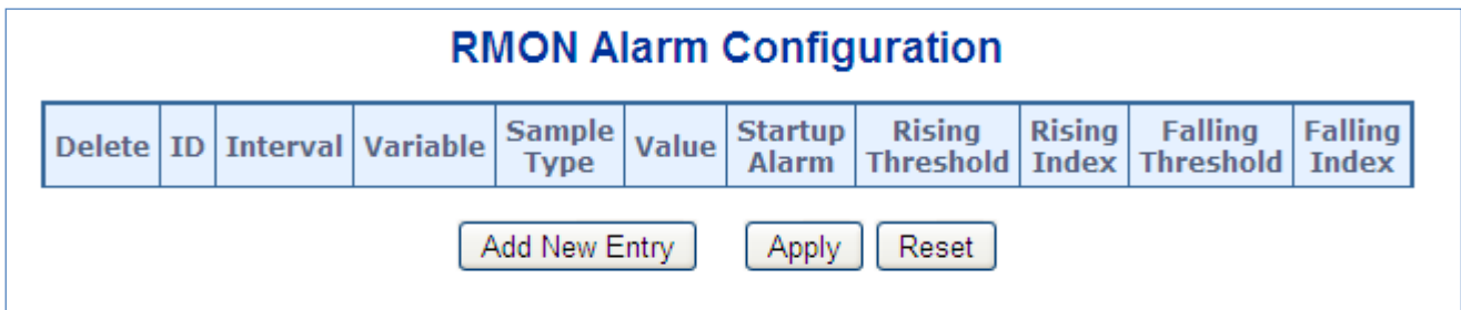
Figure 4-2-3-1: RMON Alarm Configuration Page Screenshot
