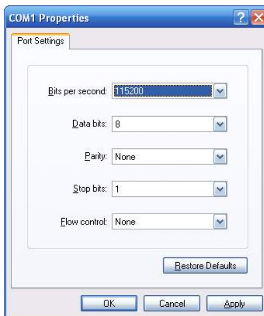
Figure 3-1-2: Terminal Parameter Settings
