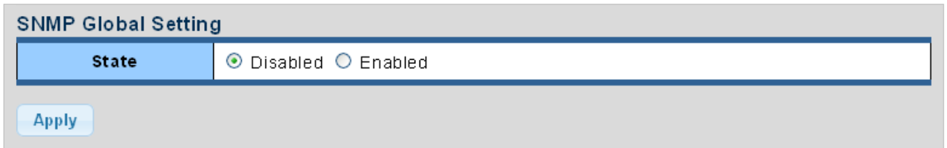
Figure 4-2-21: SNMP Global Setting Page Screenshot
