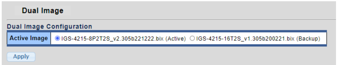
Figure 4-16-5: Dual Image Configuration Page Screenshot
