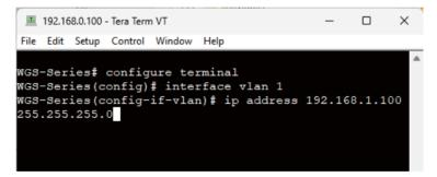
Figure 6-3: Set IP Address Command Screen
