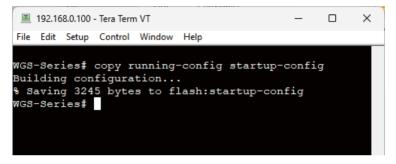
Figure 6-4: Saving Current Configuration Command Screen
