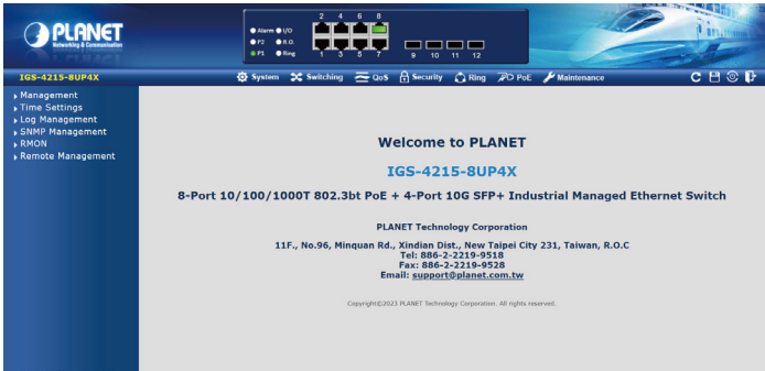
Figure 5-3: Web Main Screen of Industrial Managed Switch (Using IGS-4215-8UP4X as an representative)
